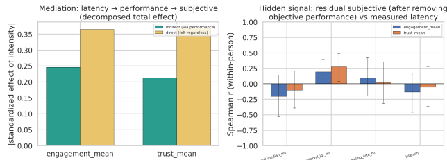
Figure 2: Left: latency’s effect on each rating decomposes into a smaller indirect path (via objective performance) and a larger direct path (felt regardless of score). Right: the residual rating, after removing objective performance within-person, does not robustly track the measured eye-tracker timing channels. Whiskers: 95% participant-bootstrap CI.
